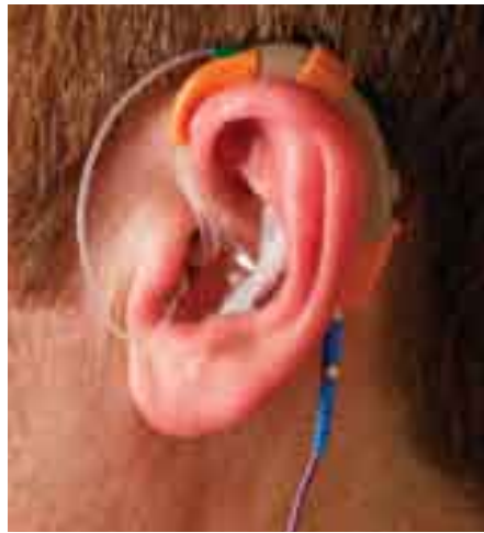
Figure 5. A recently introduced hearing aid that both measures and produces the stimuli for a real-ear measure. (Figure courtesy of Dr. Jerry Yanz of the Starkey Company.)
